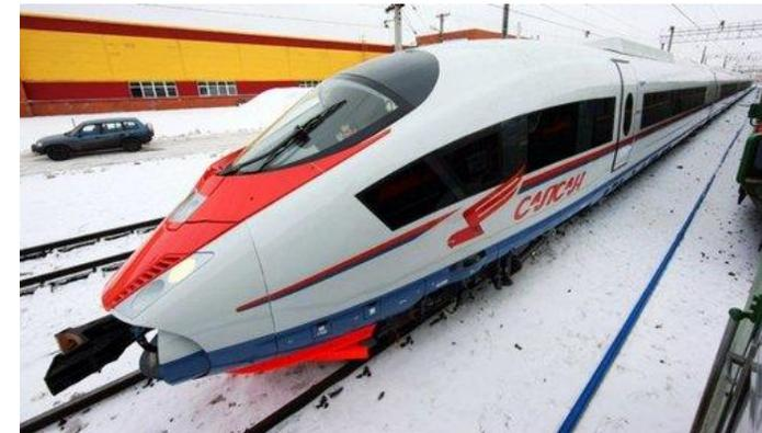
The Sapsan on the Moscow–Saint Petersburg Railway is Russia's highest speed railway with a top speed of 250 km/h (155 mph). The first upgraded 250 km/h service using Siemens Velaro RUS trains went into service on December 26, 2009.
